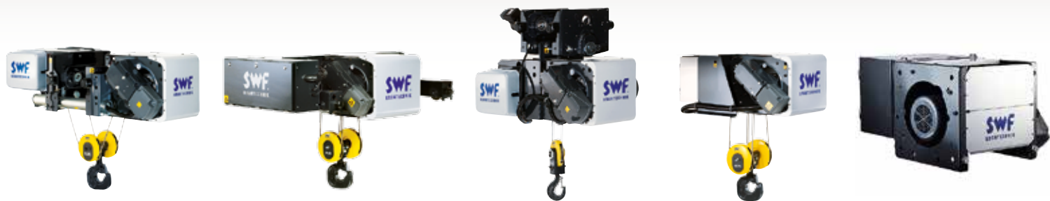
NOVA L Single girder trolley, low headroom, up to 12,5 t NOVA M Double girder trolley, up to 80 t NOVA N Single girder trolley, normal headroom, up to 40 t NOVA F Fixed hoist for free- standing installations, up to 80 t NOVA machinery hoist, up to 5 t
