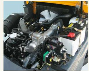
New engines, compliant with worldwide stage IIIA emission regulations
