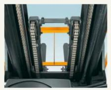
Three-stage mast with four-cylinder mechanism
