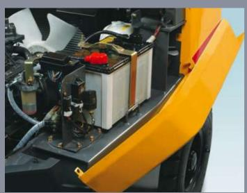
Detachable side covers for convenient inspection and simple maintenance
